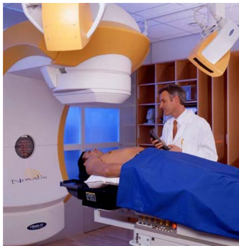
Figure 3. The custom-molded stereotactic body frame is secured to the table, precisely positioning the target in the treatment field. X-ray positioners, which are mounted on the ceiling, take stereoscopic x-rays of your anatomy and compares them to the position in the treatment planning software.
